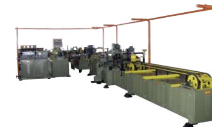
WIRE FEEDER, EXTRUDER & CONVEYOR
